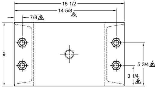
**TYPE ME-5D SPRING ISOLATORS WITH INTERNAL ADJUSTMENT**
